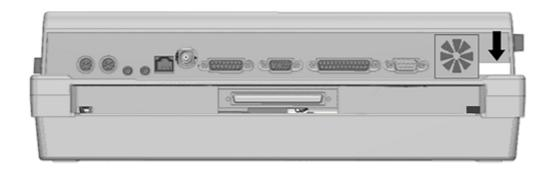
Figure 7-1. MultiBay-ISA Expansion Base Serial Number Location
